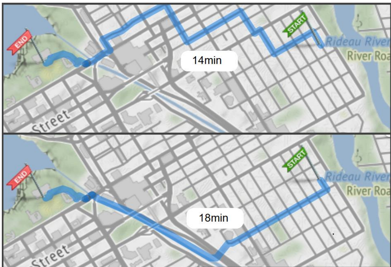
Figure 5.2 Example of the fastest and safer route found by the OTP router for a given O-D pair.
